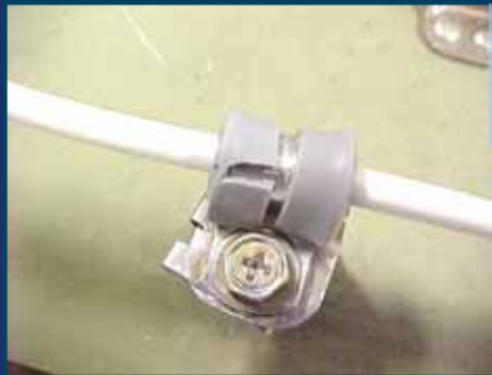
Damaged clamp cushion
