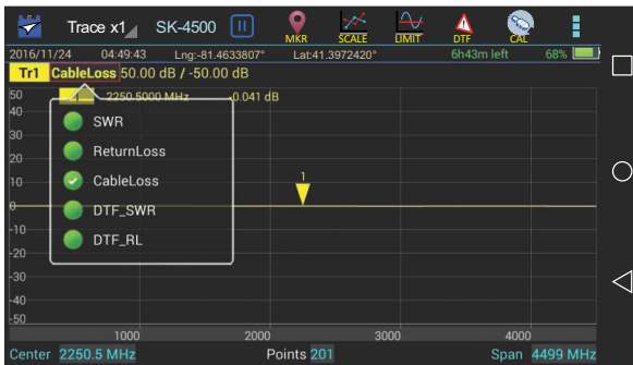
Figure 10 Selecting Cable Loss Measurement
