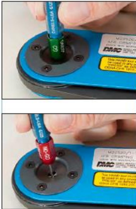
Checking tool calibration with the “GO/NO-GO” gauge
