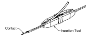
POSITION OF THE CONTACT ASSEMBLY IN THE INSERTION TOOL Figure 49
