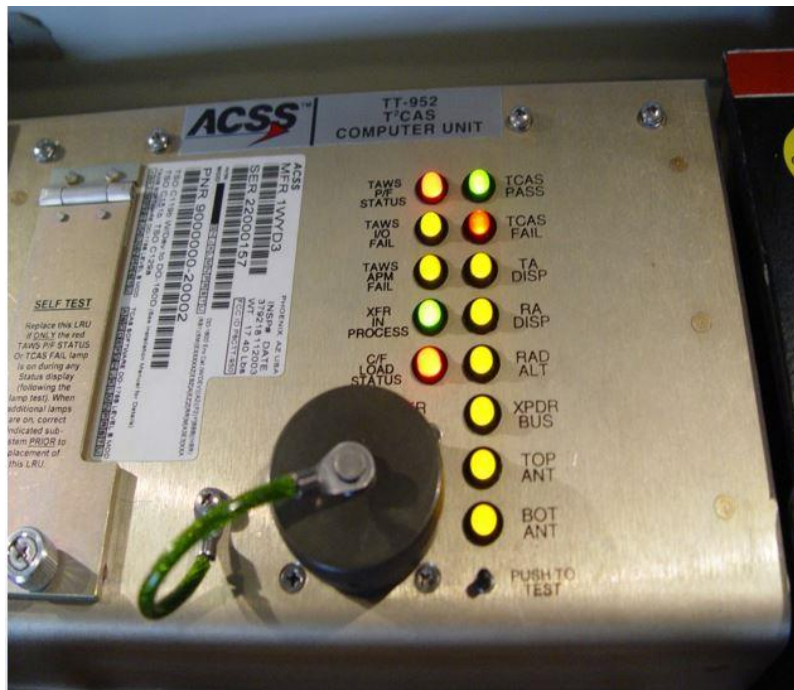
ACSS T2CAS computer with BITE capability on the front face of the box
